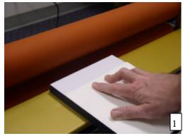
Peel release liner about 1-½" from top of coated substrate. Crease release liner.
