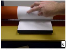
Peel off the release liner. Run the print and the substrate through the laminator. Be sure that the print does not flop down on the exposed adhesive.
