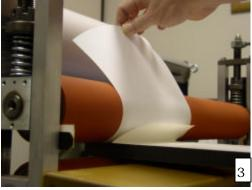
Insert tacked end of print about ½" into the laminator. (Do not catch the crease in the release liner between the rollers.) As you start the laminator, hold the print at a 45 degree angle above the top roller.
