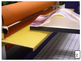
Line print up with edges of substrate. Lightly tack print along top ½" of substrate, working from the center out or from one side to the other, without trapping air. (Do NOT press along the crease in the release liner.)
