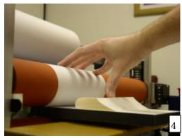
Use hand tension to wrap the print around the top roller. Make sure both edges of the print are tight against the roller to avoid trapped air and wrinkling.
